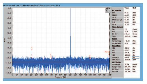
Figure 5. FFT Plot: 200 MHz Clock, 140 MHz input; SNRBOOST Disable
