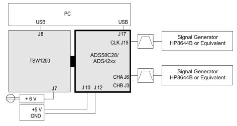
Figure 3. Test Set-up Block Diagram
