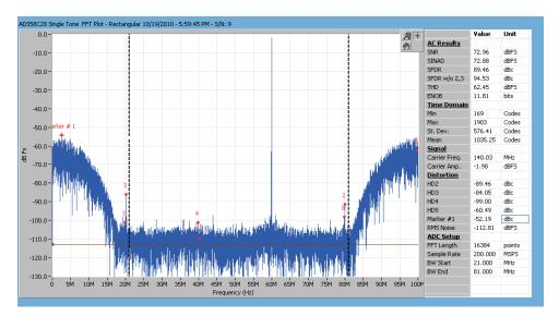
Figure 6. FFT Plot: 200 MHz clock, 140 MHz input; SNRBOOST Enabled with Filter #40 (BW 60MHz)
